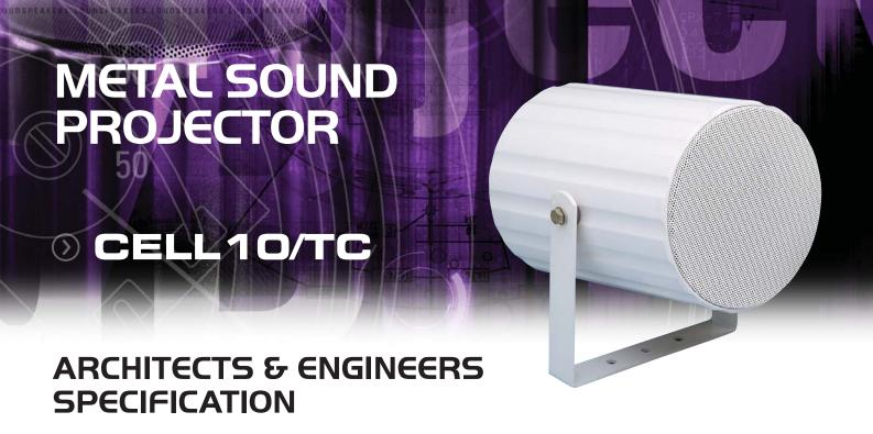
The unit shall be the PENTON model CELL10/TC or equal and approved. The speaker enclosure shall be constructed of high-grade extruded aluminium with a mesh grille, epoxy coated to match the enclosure. The mounting will be via a "U" shaped aluminium bracket. The speaker assembly shall comprise of 130mm dual cone loudspeaker.
