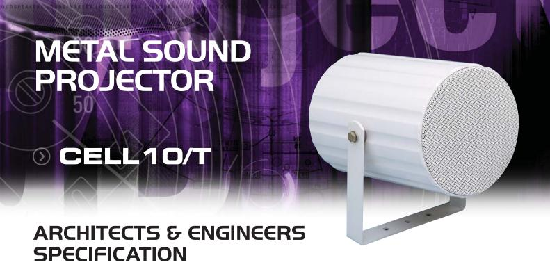
The unit shall be the PENTON model CELL10/T or equal and approved. The speaker enclosure shall be constructed of high-grade extruded aluminium with a mesh grille, epoxy coated to match the enclosure. The mounting will be via a "U" shaped aluminium bracket. The speaker assembly shall comprise of 130mm dual cone loudspeaker.
