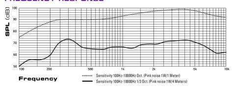
The RCS8FTCX/EN & ENC have been tested for 100 hours at a maximum power of 20W. Both units did not deviate by more than +/3dB. The frequency response and impedance curves remained constant throughout the test period. All results are in full compliance with the requirements of EN54-24.
