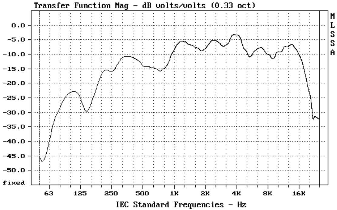
Note: The wide band frequency response is derived using MLS methods and does not necessarily relate to the sensitivity values given in the summary table.
