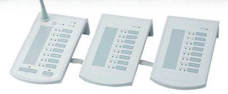
PPM-AS/PSM is an unidirectional addressable condenser paging microphone for the IDA8 and DIVA system. In accordance with BS5839, it is monitored by using RS485 protocol over STP CAT5/6 cable, and transmits both audio and power from the paging console to the system units. The PPM-AS/PSM has 8 zone buttons with a sleek gooseneck microphone, providing durability and aesthetics in a slim, stable chassis.
