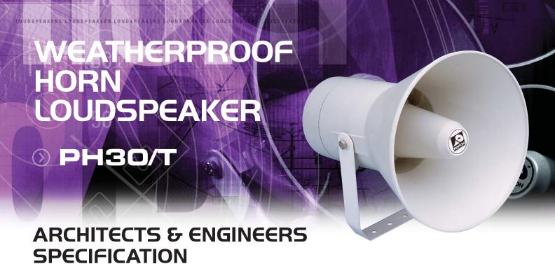
The unit shall be the PENTON model PH30/T or equal and approved. The horn enclosure shall be constructed of high impact ABS with UV inhibitors and non-perishable gaskets to prevent the ingress of water or dust and be rated to a minimum of IP66. The unit will be mounted via a stainless steel "U" bracket and fixings. The speaker assembly shall comprise of a high-density phenolic resin diaphragm housed in a flared chamber, 287mm long x 238mm diameter.
