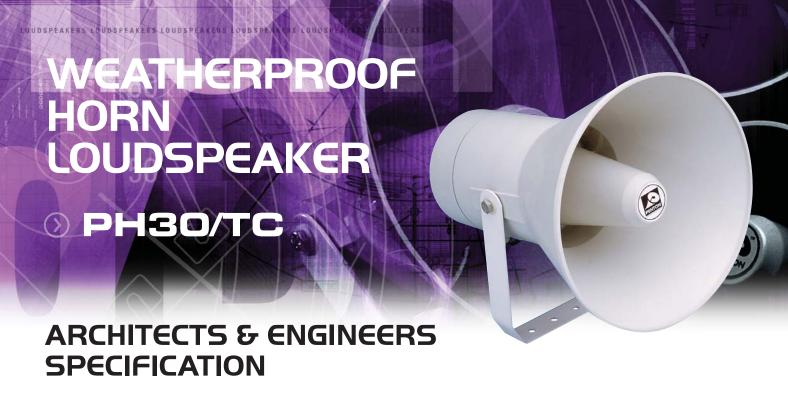
The unit shall be the PENTON model PH30/TC or equal and approved. The horn enclosure shall be constructed of high impact ABS with UV inhibitors and non-perishable gaskets to prevent the ingress of water or dust and be rated to a minimum of IP66. The unit will be mounted via a stainless steel "U" bracket and fixings. The speaker assembly shall comprise of a high-density phenolic resin diaphragm housed in a flared chamber, 287 mm long x 238 mm diameter.
