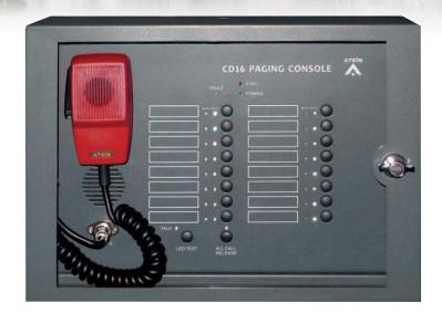
The CD-16 paging console is a remote paging interface with Access Level 2 protection in compliance with EN54-16. Compatible with DIVA8 and IDA8 PAVA systems, the unit serves up to 16 zones individually with an All-Call option. Zone selection buttons and fireman's fist microphone are encased in a heavy-duty IP30 wallmount metal box with lockable door.
