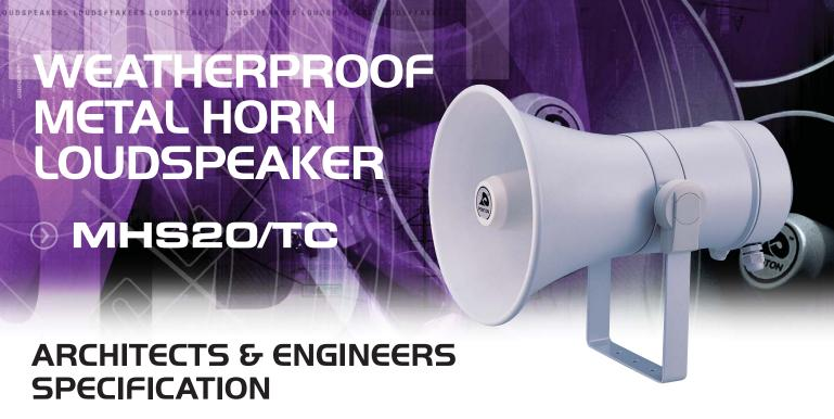
The unit shall be the PENTON model MHS20/TC or equal and approved. The horn enclosure shall be constructed of a weather-resistant, LM4 aluminium die-cast housing incorporating a rear chamber. The unit will be mounted via a lockable, stainless steel "U" bracket and fixings. The loudspeaker diaphragm shall comprise of a high density phenolic resin type capable of withstanding water and dust ingress up to a minimum IP65 Norms housed in a flared chamber, 297mm long x 217mm diameter.
